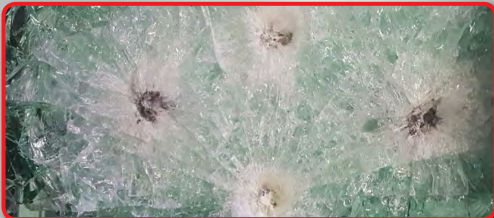
ANTI-BANDIT DOORS & BULLET PROOF PANELS AK47, 7.62 X 39 API, 4 SHOTS FROM 30M
